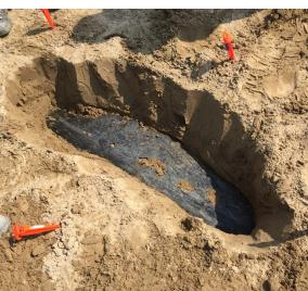
Example of superficial damage hidden underneath a sandbag, detected through the sack during a water pudde test.
