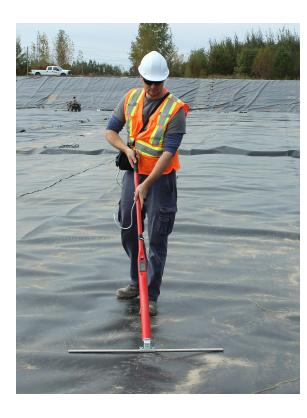
Different equipment can be used depending on the area to be surveyed. Small hand-held detectors are used in confined areas, whilst large detectors are generally used on expansive open areas. Leaks of less than 1 mm<sup>2</sup> can be localized using the spark test method.
